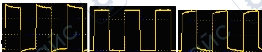
Overcompensated Compensated correctly Under compensated
